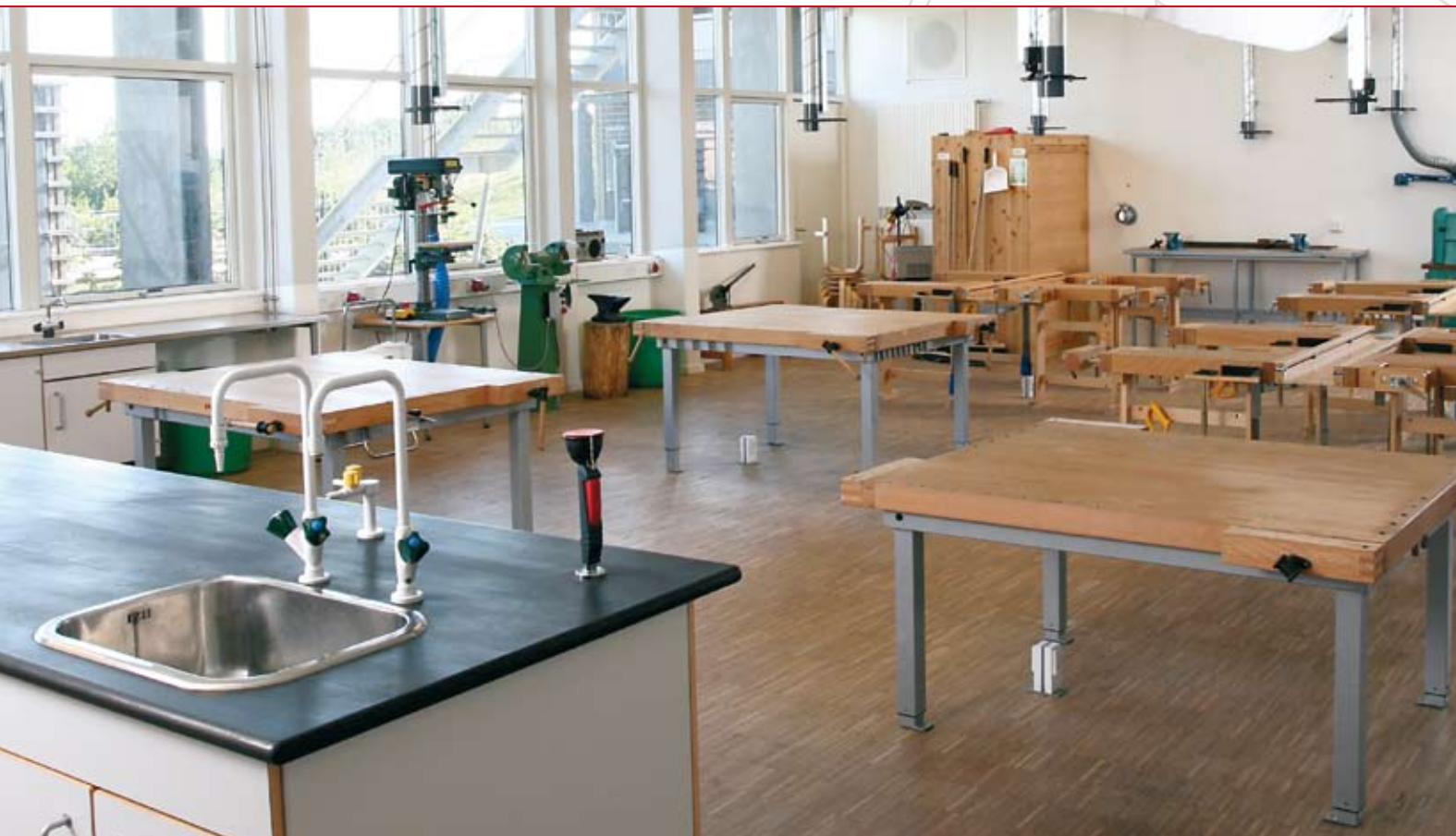
▲ Teacher desks can be equipped with sink, gas, electricity and emergency shower if required, thus making it possible to interchange technology subjects with other subjects such as science. The combination of traditional work benches and four-sided, height adjustable technology benches make the room very flexible.
