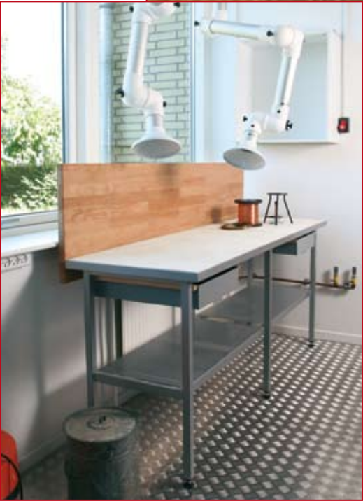
▲ Working table with fire resistant stone plates on the table top. For soldering or welding purposes, extraction is necessary.
