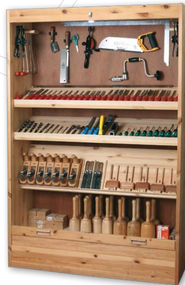
▲ The ST standard tool unit containing a complete tool set is the minimum amount of equipment in every wood-working room. The unit is lockable, naturally.
