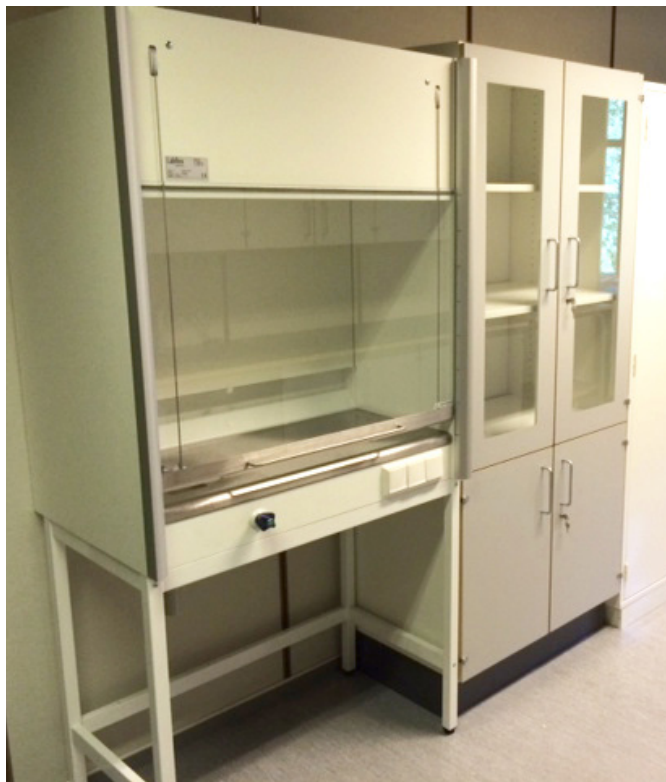
Example: Fume hood installed on a worktop frame
