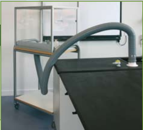
▲ Mobile extraction hoods facilitate flexible demonstration.
